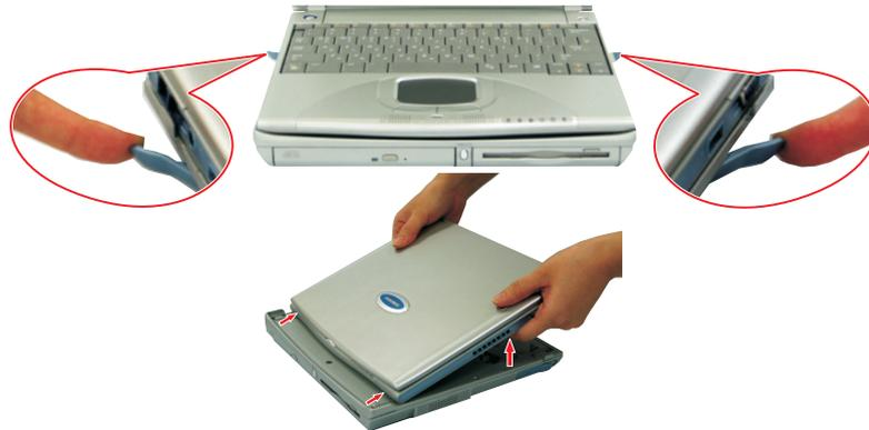
5. After tilting remove the system by sliding/lifting out toward the back of the docking station.
