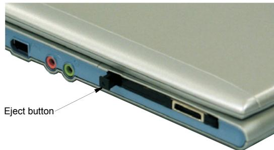
3. Push the eject button once to pop it outward then push the eject button again to eject the card.
