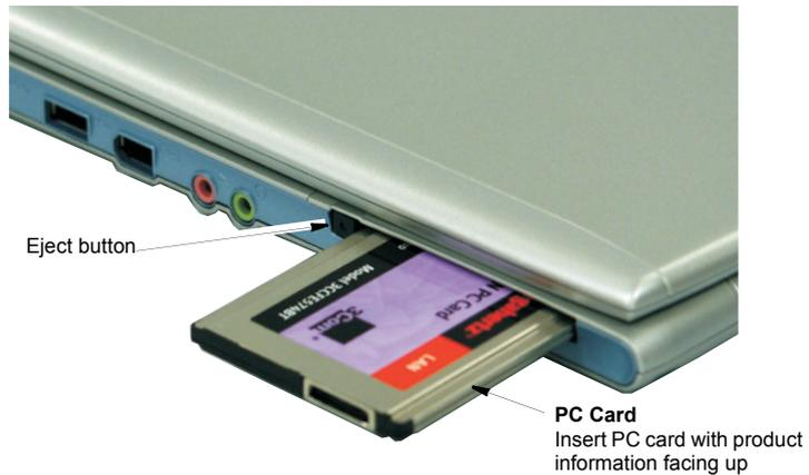
Windows automatically assigns computer resources (such as communication ports and memory addresses) to the PC Card installed in your computer.
