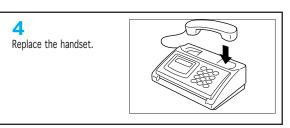
■ The machine begins receiving and returns to Standby Mode when reception is complete.
