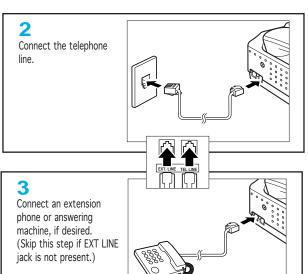
Plug one end of the telephone line cord into the TEL LINE jack and the other end into a standard telephone wall jack.
