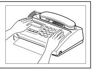
✓ Press down on the cover using both hands until it snaps into place.
