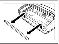
Carefully pull out the jammed paper in the direction of arrow.
