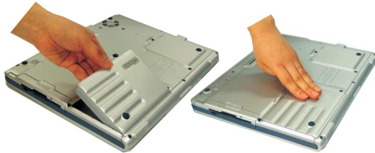
2. Place the battery inside and against right side of the computer battery compartment at an angle of approximately 30 degrees.
