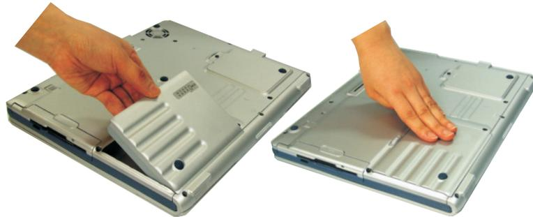
2. Place the battery inside and against front side of the computer battery compartment at an angle of approximately 30 degrees.
