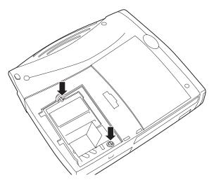
Grasp the pull tab and lift out the lamp module.
