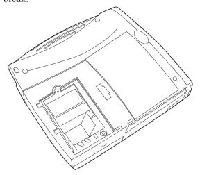
7. Install the new lamp module, being sure to align the connectors properly.
