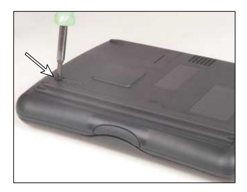
${f 5}$  Slide the battery release latch to release the battery.
