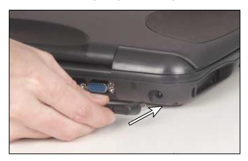
The battery charging indicator light turns on. If the battery charging indicator light does not turn on, disconnect the adapter from your notebook and repeat Step 2.
