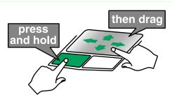
Position the pointer over the object. Press the left button and hold it down, then use the touchpad to move (drag) the object to the appropriate part of the screen. Release the button to drop the object where you want it.
