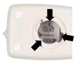
Replace the mouse ball and lock the retaining ring into place.
