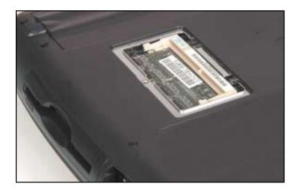
5 If you are removing a module, gently press outward on both clips at either end of the memory module until the module tilts upward.
