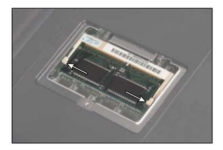
6 Pull the memory module out of the slot.
