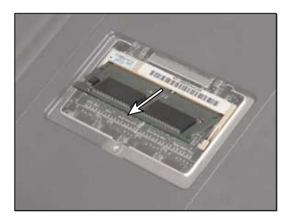
**7** Hold the new or replacement module at a 30-degree angle and slide it into the empty memory slot.
