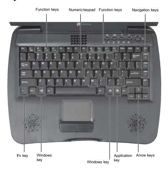
Your notebook features a full-size keyboard that has the full functionality of a desktop computer keyboard. Many of the keys have been assigned alternate functions, including shortcut keys for Windows, function keys for specific system operations, and the Pad Lock keys for the numeric keypad.
